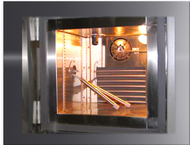
The ELH Calibration Chamber with probes inserted through access port.
